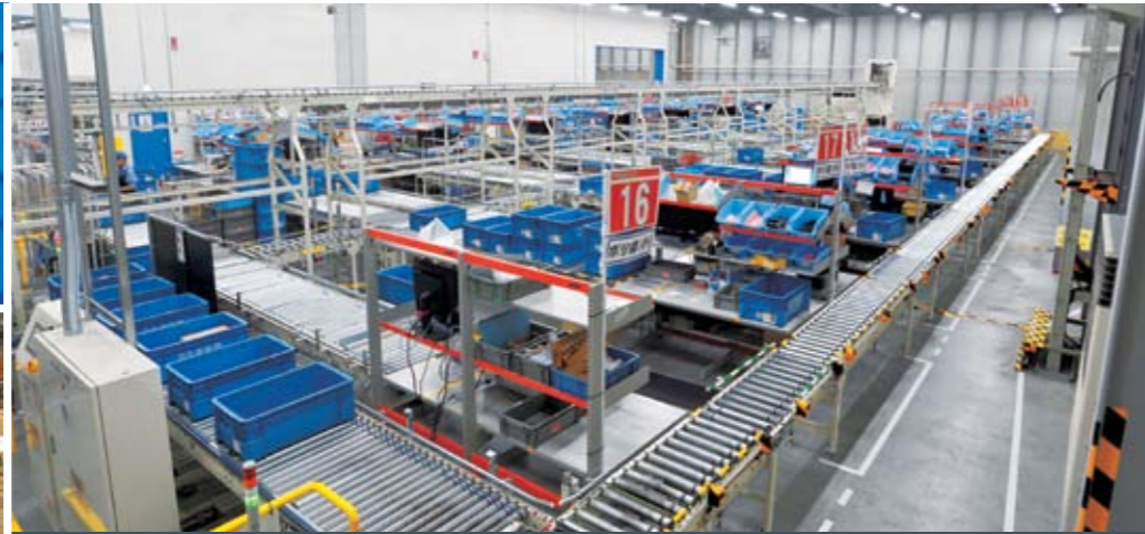
Small parts bearing information such as name, quantity, weight and date that are translated into bar codes are kept in a fixed location. Automatic input of data and reading improves efficiency. The ordered parts in each blue box are separated on the conveyor belt automatically.
