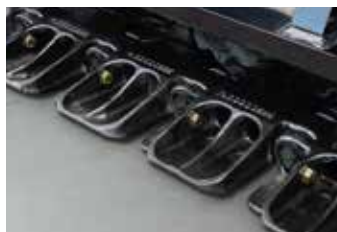
High-durability box type track shoes Lower rollers with 20% greater contact width
