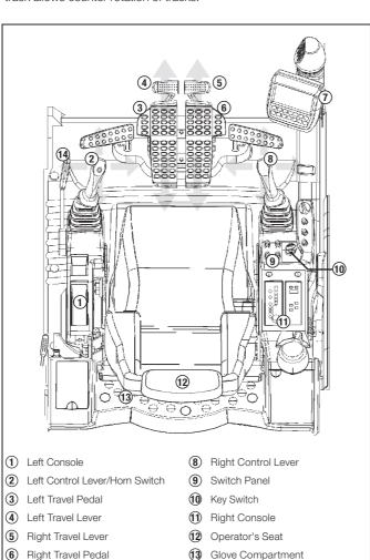
14 Pilot Control Shut-Off Lever
