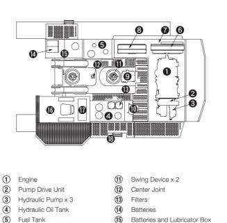
**(6)** Engine Radiator (7) Engine Air Cooler
