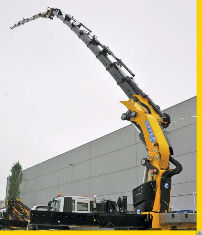
In the design stage of a truck-mounted crane, the crucial element in providing exceptional solutions is the **second boom** and its junction with its relative extensions.
