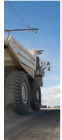
Trolley-assisted dump trucks achieve significant fuel savings, reduce CO<sub>2</sub> emissions and improve productivity. They also allow trucks to drive uphill faster than they could using diesel engines. This is made possible by receiving electric power from overhead contact lines powering their AC motors (instead of the truck’s diesel engine). Find out more on page 16.
