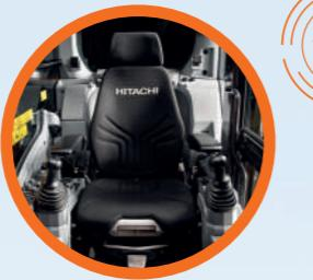
Vibration in the cab is reduced by up to 27% during travelling and heavy-duty operation thanks to new viscous mounts providing optimum suspension.
