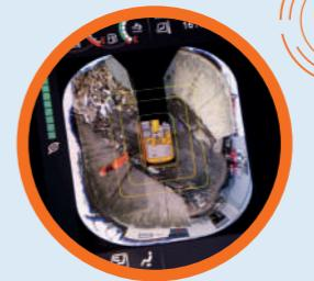
Visibility is excellent thanks to the Aerial Angle camera system, new LCD monitor and new parallel wiper.
