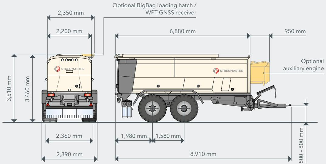
MACHINE TRANSPORT SW 218 TC - TIRES REMOVED
