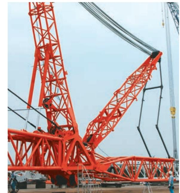
**Hydraulic type rear post back stop with self-powered assembly and storage device (with luffing specifications)**
