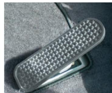
**Hydraulic slewing brake pedal is standard**
