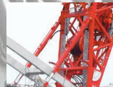
**Hydraulic cylinder type boom back stop**
