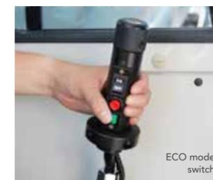
Fuel economy has been improved drastically when winching up and down with light loads. This design ensures energy-efficient operation over repetitive movements or working with loads at heights.
