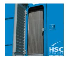
**Separated oil cooler from engine radiator**
