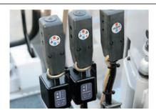
Control levers of two main and boom hoist drums each fit the drum rotation knob vibration during inching lever
