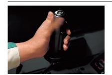
**One -hand acceleration grip** Thanks to a unique grip design, an easy -precise-minute control of engine rpm and pump discharge from min. thru max. is really possible at the same time by simply twisting the grip fitted on slewing control lever.
