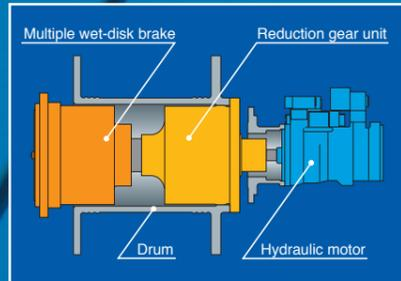
**Advanced clutchless multiple wet-disc brake is well designed, and ensures continuous heavy-duty operation.**
