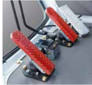
Winch with free-fall function (brake pedals)
