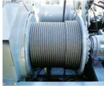
Drum with integrated reduction gear (winch with free-fall function)
