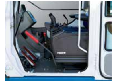
A gate lock lever keeps the crane safe against accidental operations
