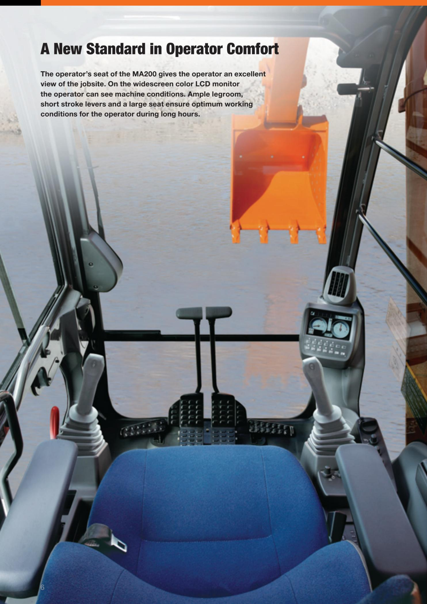
The MA200 cab has been redesigned to meet demands of customers. From the operator's seat the operator has an excellent view of the jobsite. On the widescreen color LCD monitor the operator can see machine conditions and with the rear view camera, what is behind the machine. Ample legroom, short stroke levers and a suspension seat with heating ensure optimum working conditions. The seat features horizontal, vertical adjustments and has a backrest contoured for comfort, with a HITACHI logo.
