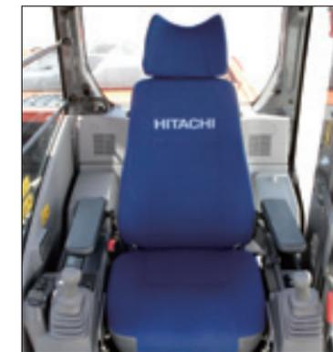
Wide adjustable armrests and a retractable seat belt are included. Short stroke levers allow for continuous operation with less fatigue. Three switches on the lever (optional) can be set to operate attachments other than buckets. The cab is pressurized to keep out dust. Noise and vibrations are kept to a minimum due to the elastic mounts, filled with silicone oil, the cab rests on.
