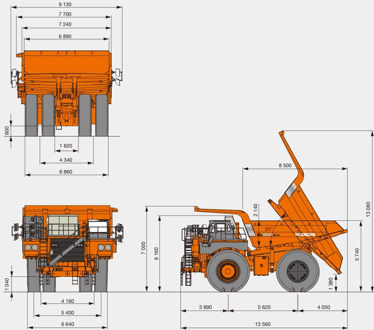
Note: Dimensions shown are for an empty machine with 37.00R57 tires.
