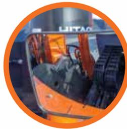
Slide cab rear mirror for safe operation of the sliding cab.
