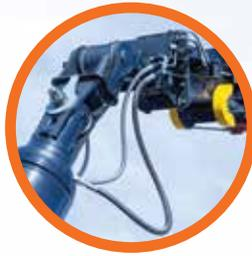
Increased versatility with rotation piping enables work with swivel clamshell buckets.
