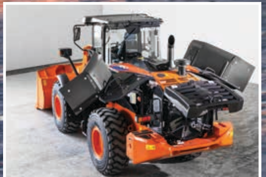
Easy access for maintenance from ground level.
