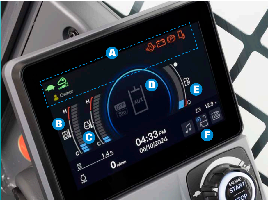
A. Machine Status Indicator (such as working function, battery charge indicator etc.) B. Hydraulic Oil Temperature C. Coolant Temperature D. AUX Mode E. Fuel Level F. Menu Icons
