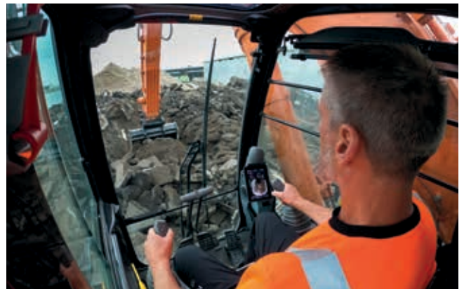
Wide view wiper design provides greater visibility.
