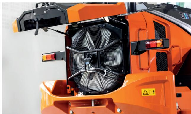
Intelligent fan operation system prevents radiators clogging.
