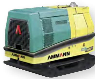
The APH 1000 TC is an IR remote-controlled hydrostatic plate that can go where others can't. The IR remote abilities ensure operation under the toughest conditions – and in the tightest spaces and deepest trenches. The operator is able to steer the vibratory plate from a safe distance with a remote control or cable remote.
