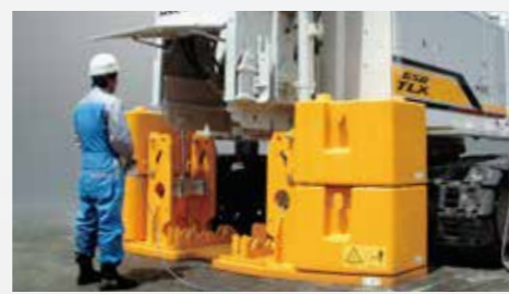
Counter weight with self-assembly unit OPTION
