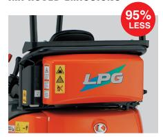
Compared with diesel engines, thanks to its clean-burning propane engine, the Kubota Mini Excavator emits almost zero PM and reduces NOX and HC emissions to just 5% compared to a diesel engine.
