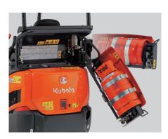
Depending on the working environment, one LPG tank can last an entire working day. Unlike diesel fuel, LPG can't spill and contaminate the surrounding environment. A hard cover protects the tank from direct sunlight and other objects.
