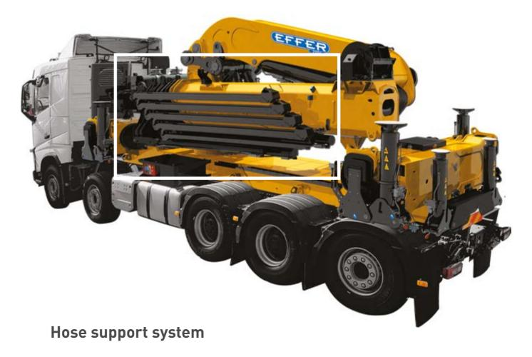
Effer offers a mechanical hose support system as well that ensures the maximum robustness.
