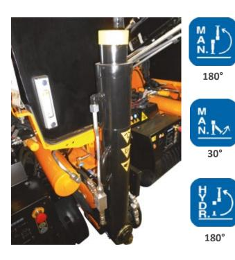
1. Short arm (C version) Versions C3s and C4s allows you to work near to the truck side with a greater distance between the hook and the ground. This allows you to have more space in that area.
