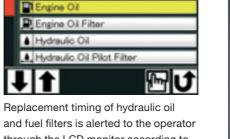
and fuel filters is alerted to the operator through the LCD monitor according to the schedule preset by the user each time when turning the key switch. The scheduled maintenance can prevent the failure of the machine.
