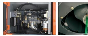
Wide doors give access to the fuel filter, water separator and engine oil filter. A large handrail, steps and anti-skid plates lead to the engine cover. The engine oil pan is fitted with a drain coupler. When draining, an associated drain hose is connected to the drain coupler. The drain coupler is reliable, avoiding oil leakage and vandalism.
