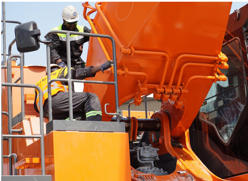
■ Assembly of excavator booms at the MECET factory in Dubai.
